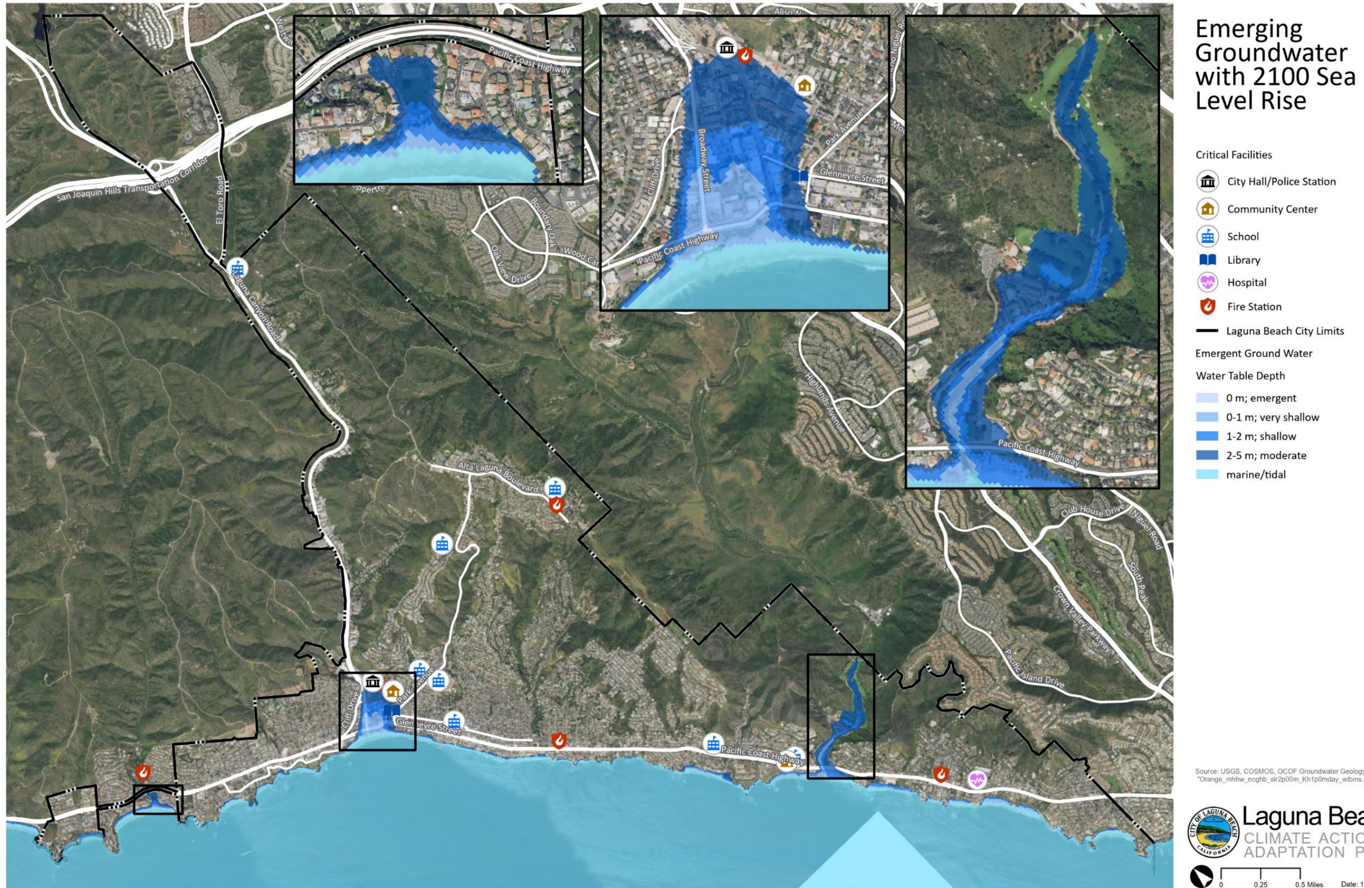
Figure 12: Emergent Groundwater Due to Sea Level Rise in 2100
